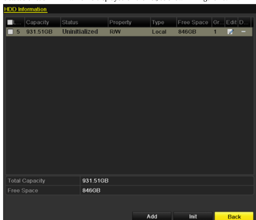
Figure 10. 17 View HDD Status (1)
